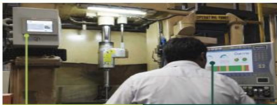
Device collecting data on legacy machines
